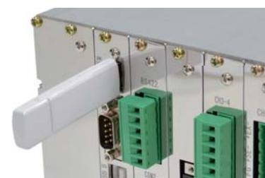
The USB host port is installed in CPU substrate of this unit. Data between PC can be handed over by using USB thumb drive. When maintaining it, it can back up data, and the program can be updated.
